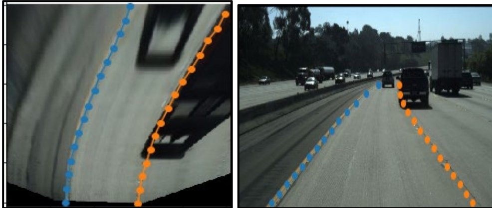
Figure 5. Final Result Visualization after Curve Fitting and Inverse Projection Mapping
