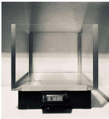
Figure 1. Apparatus used for the hot plate test.
