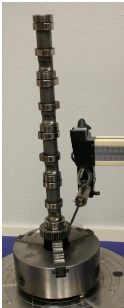
Fig. 1. Camshaft circular runout measurement
