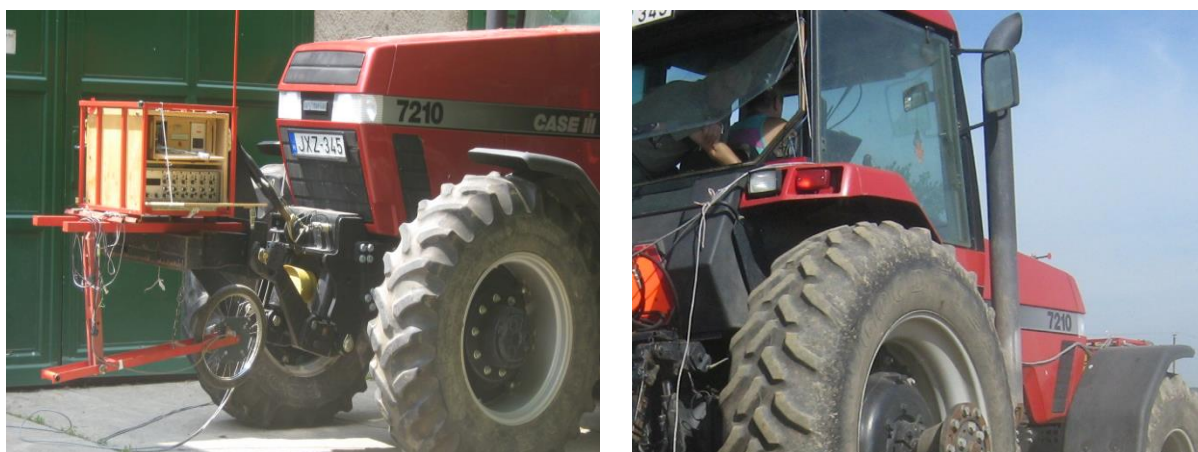
Fig. 1 CASE IH 7210 tractor with Paraplow tools and with Computer
