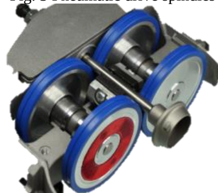
Fig. 5 Mechanic drive spindles whit twin Disc.
