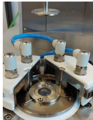
Fig. 4 The placement of the MR fluid in the viscometer
