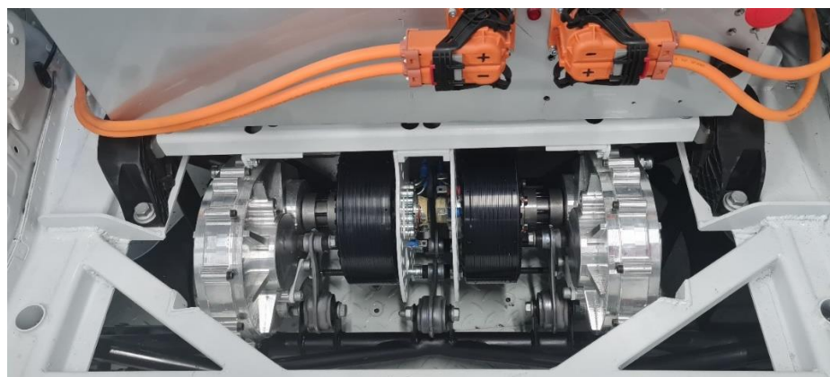
Fig. 2 The original solution of rear powertrain E-up Boost
