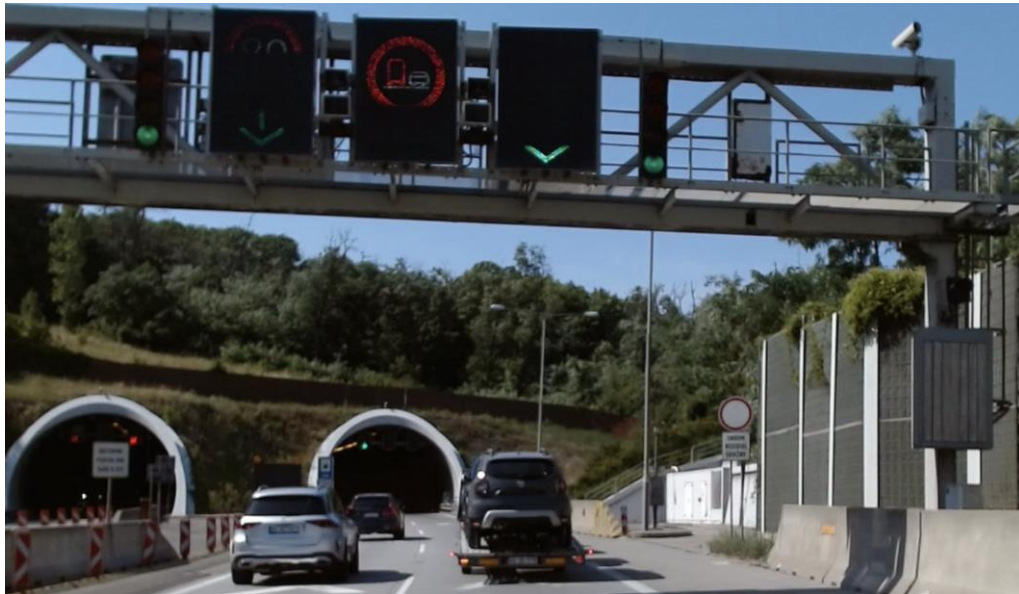
Fig 8: Example of unreadable digital signs in the single frame because of the sign refresh rate.
