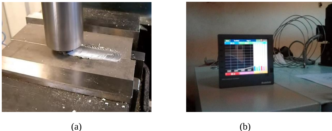
Fig. 2 a) Fiction Stir Welding of AA5052-AA6061 plates with a conventional milling machine. b) Temperature – time measurement with data acquisition.
