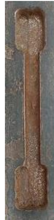
Fig. 2 I-section machined En 31 material
