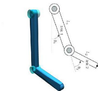
Figure 2. 2 Degrees of Freedom exoskeleton designed in Autodesk inventor software.
