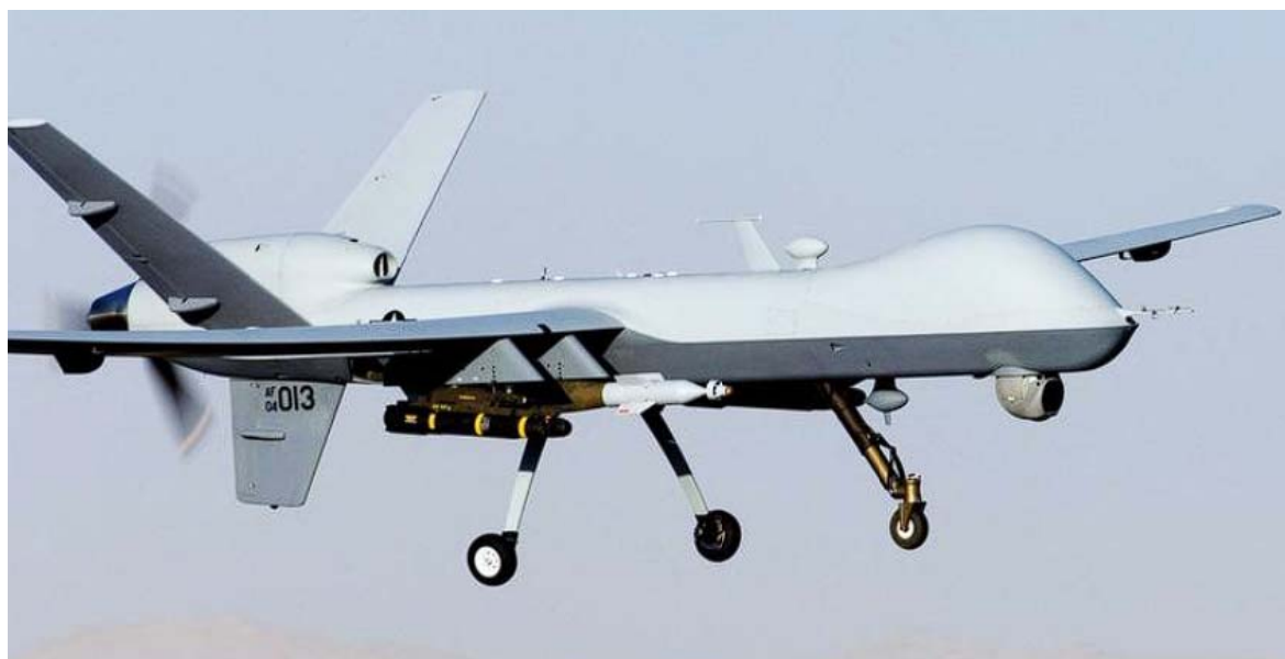
Figure no. 1: MQ-9 Reaper drone with Hellfire missiles and JDAM bombs (Source: Sherman, 2023)
