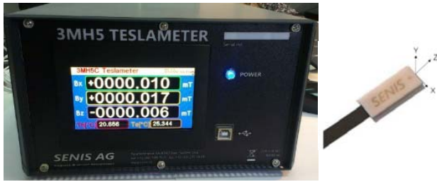
Fig. 1. SENIS Low-Noise Teslameter 3MH5 and Hall probe C.
