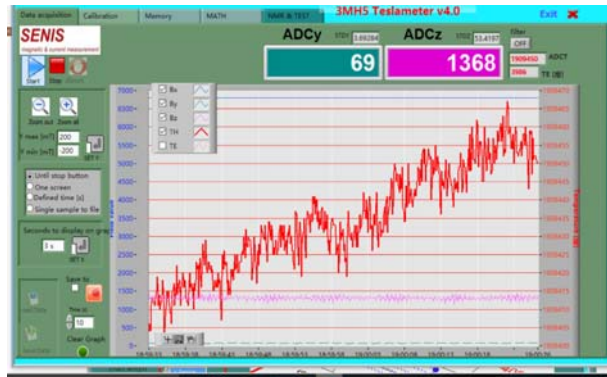
Fig. 13. Drawing curves of magnetic induction intensity and temperature values.
