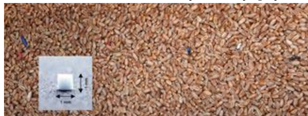
Fig. 8. Encapsulated beryllium oxide dosimeters (blue, red, white) in a batch of cereal seeds (large image). Blank 1 mm dosimeter (detail picture).
