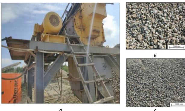
Fig. 5 General view of PULVOMATIC series crusher model 1145 (a), raw material (b), and finished product (c)
