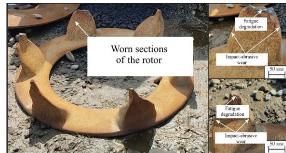
Fig. 6 Character of catastrophic wear of the rotor of the PULVOMATIC series crusher model 1145
