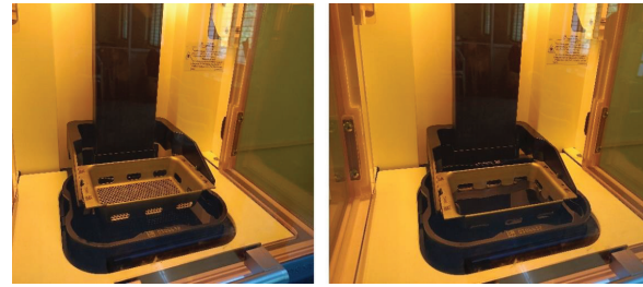
Fig. 6. Bottom-up approach 3D printing of pallet coupons in DLP method
