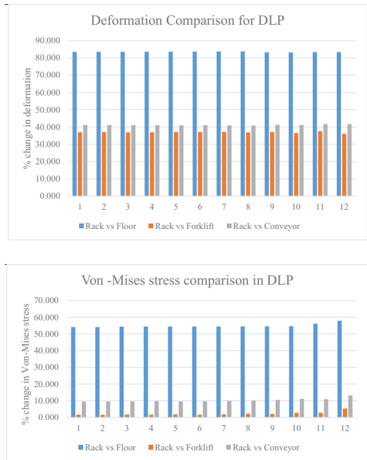
Fig. 26. Comparisons of deflection and stresses for DLP-manufactured pallet
