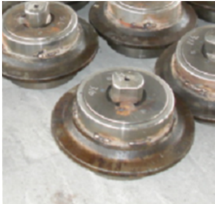
Fig. 5. Disk cutter with normal wear dismantled on site
