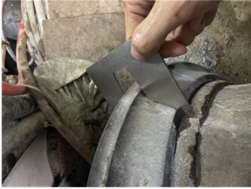
Fig. 8. Disk cutter wear values were measured on site
