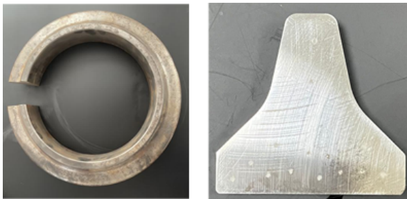
Fig. 10. Normally worn disk cutter ring and test piece
