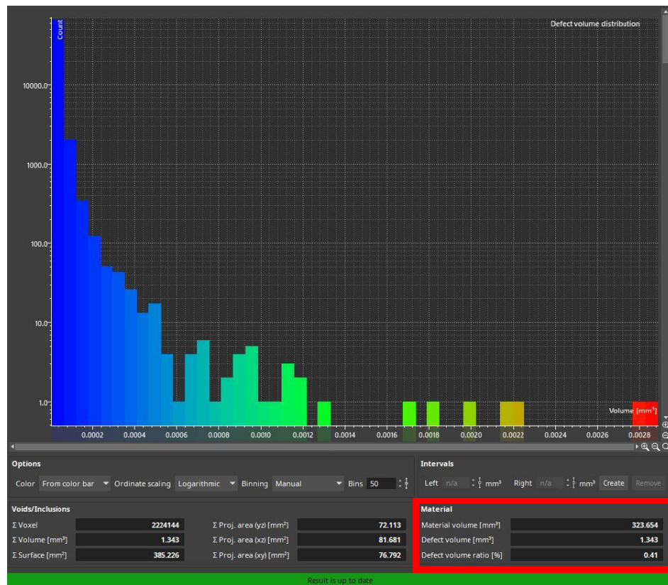
Fig. 5. Results of statistics on the analysis of the porosity (number of pores by volume) of a specimen with a honeycomb structure; statistics circled in red frame
