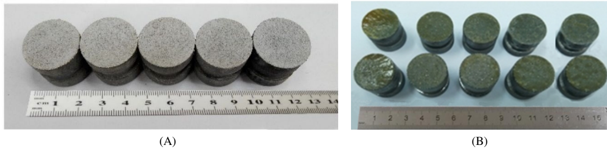
Fig. 10. Specimens of 3D-printed titanium substrates with HA microplasma coating before (A) and after (B) tensile adhesion tests. HA, hydroxyapatite
