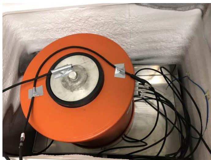
Fig. 3. Photograph of the sample assembly placed in the freezer with temperature sensors connected.
