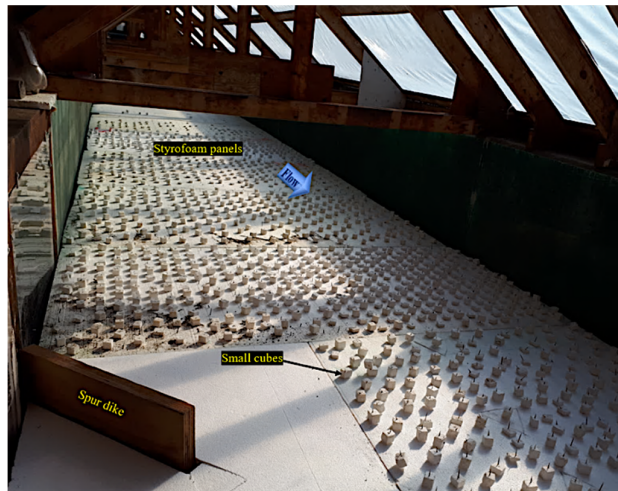
Fig. 2. A cover condition experiment under smooth ice cover with a 45° inclination angle.
