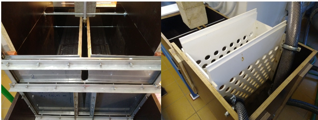
Fig. 2. TPW and adjustable sidewalls (left), flow straightener (right).
