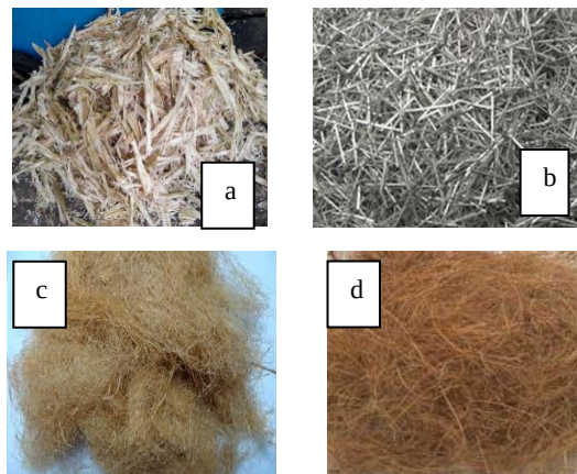
Figure 1. Different types of Fibers: a) Sugarcane Fiber, b) Steel Fiber c) Bamboo fiber, d) Jute fiber
