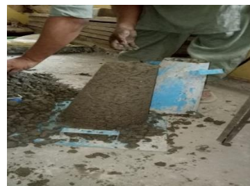
Figure 4. Performing Slump Test
