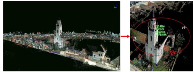
Figure 14. The 3D point cloud image of the church and automatic height measurements of objects
