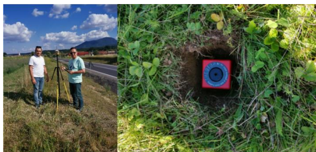
Figure 7. The GNSS mount on the base point (left image) and marking the points on the ground using Feno type survey marker
