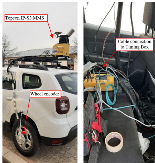
Figure 3. The mounting MMS on a 4x4 SUV, wheel encoder, and cable connections to the timing box inside the vehicle
