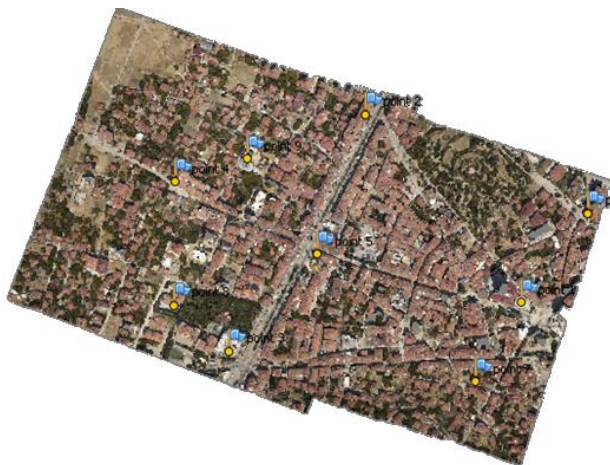
Figure 6. Ground control points selected from LiDAR point cloud
