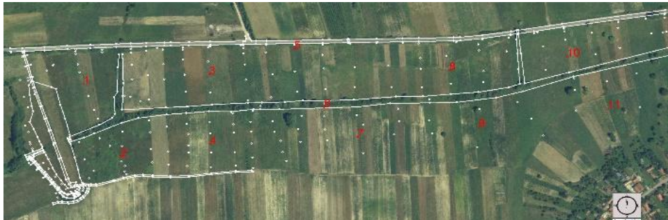
Figure 2. Botean II polder – distribution of measured points (Dataset, white colour) and control points (red colour)
