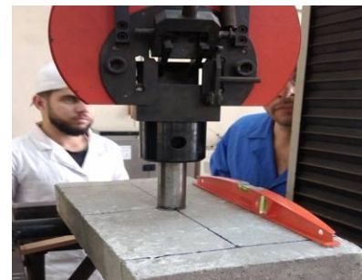
Figure 10. Centered punching test
