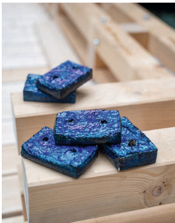
III.2. Brick from mycelium - circular contact - brick project by Anna Maria Wierzbicka. Production and firing - Łukasiewicz Institute in Łódź. photo: Artur Brzozowski
