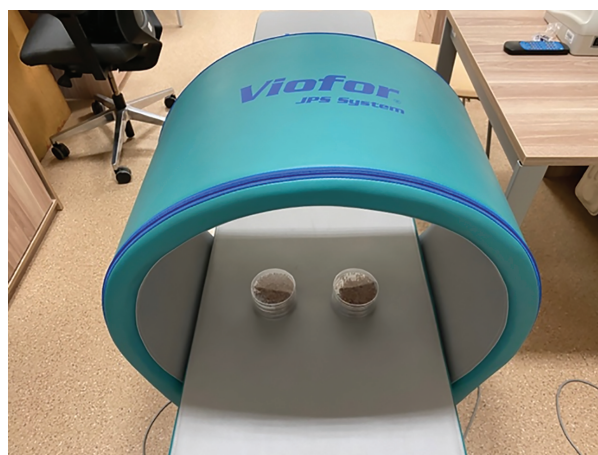
Figure 1. The radish seeds in Petri dishes in the Viofor JPS Delux machine used in the experiment to generate LFMF.
