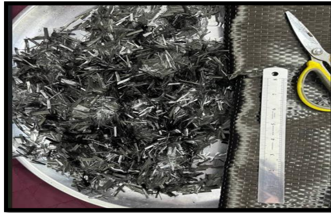
Figure 2: Carbon fiber before and after cutting into a specific length
