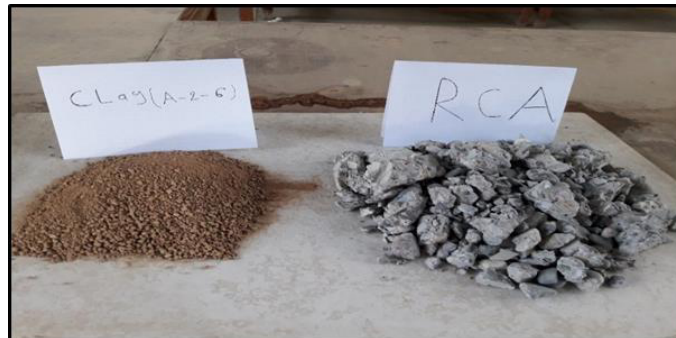
Fig. 2: Shows the recycled aggregate and the used clay soil
