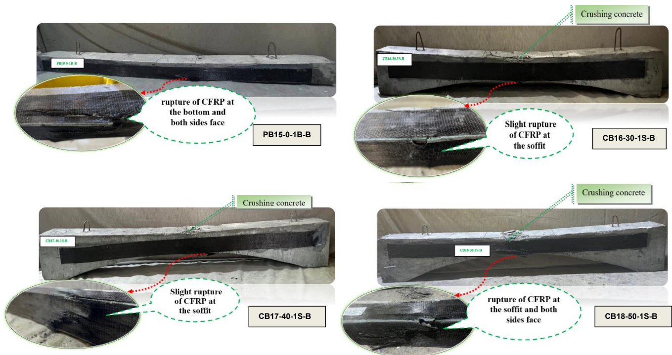
Fig. 12: Cracks pattern and failure mode of G5
