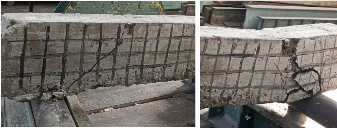
Fig. 3: Shear Crack pattern in HSC
