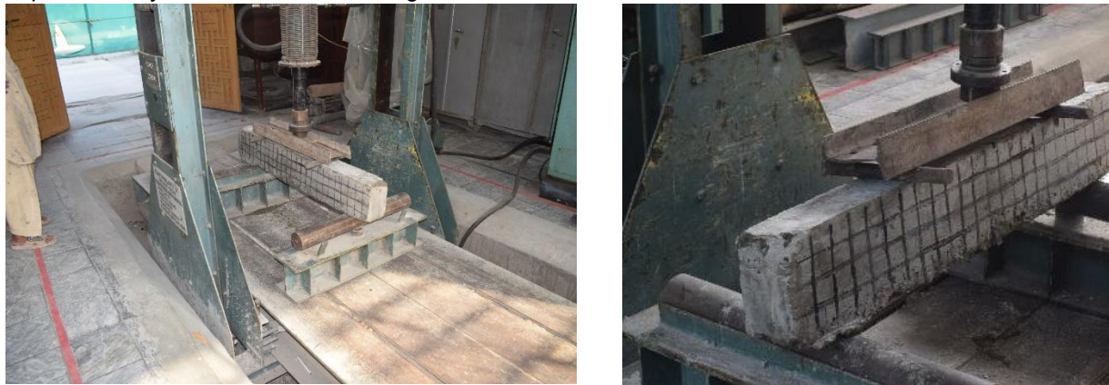
Fig. 2: Testing Setup of HSC Beam
