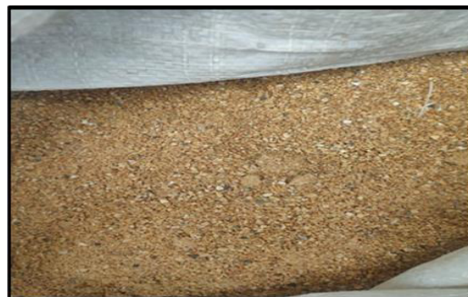
Fig. 2: Crushed alumina bricks as fine aggregate
