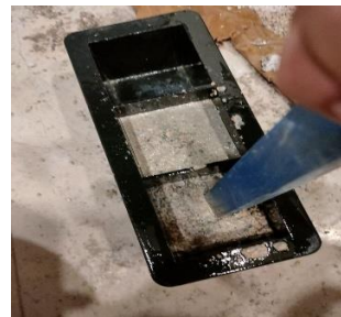
Fig.6: By using a tiny steel hammer to compacts specimens.
