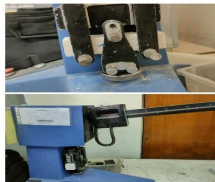
Fig .14: Modulus of rupture testing mechanism.
