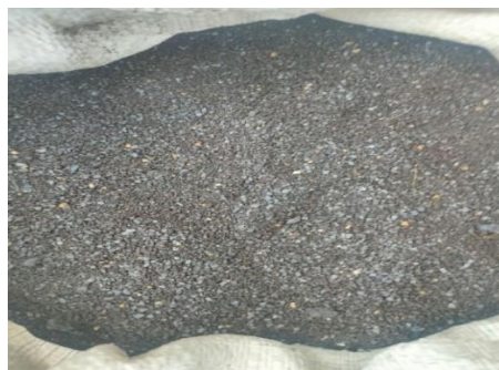
Fig.3: Crushed magnesite bricks as fine aggregate
