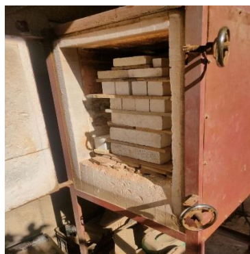
Fig.7: Preheat the oven to 1000°C and 1100°C while the models are inside.
