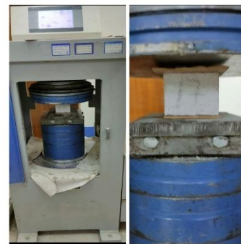
Fig.12: Compressive strength testing mechanism.
