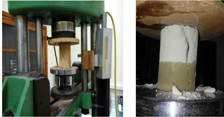
Fig. 3: Experimental Material for Dry and Wet Compressive Testing
