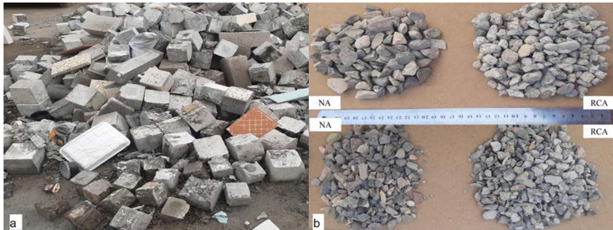
Fig. 2: Recycled coarse aggregate preparation: a) Tested concrete specimens that were discarded, b) Natural and recycled coarse aggregates after sieving.
