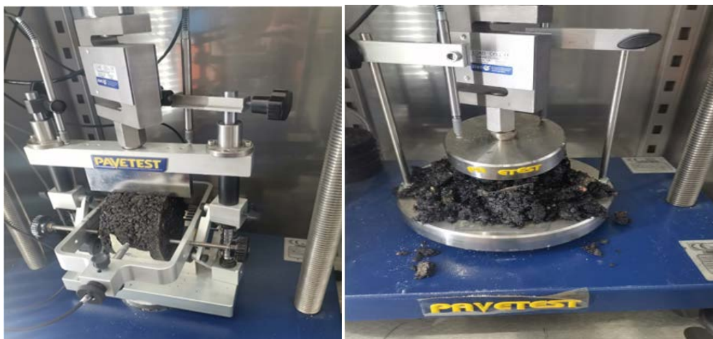
Fig. 7: a) Resilient modulus test, b) Sample under dynamic creep test.
