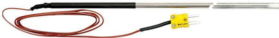
Fig. 11: AK probe thermocouple. Taken from Benedetto et al. [35].
