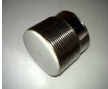
Fig. 12: A typical ice sensor. Taken from Troiano et al. [37].
