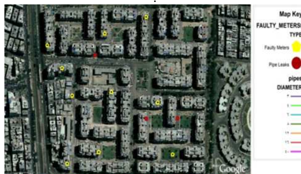
Fig. 8: Pipe leaks and faulty meters locations over Google Maps using ArcGIS.
