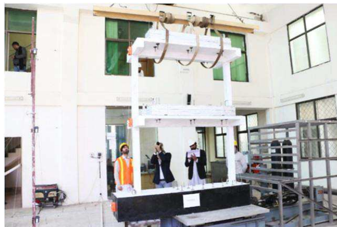
Fig. 4: 1/3rd reduced RC frame model setup.
