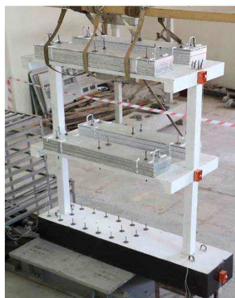
Fig. 3: Extra weights in the form steel plates for seismic mass modeling.
