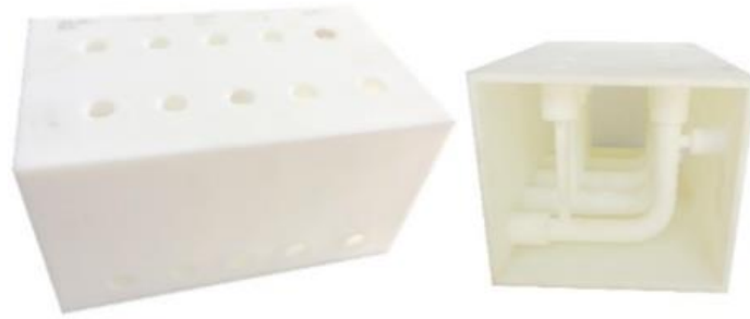
Fig. 3 – A manifold using stereolithography (SLA) built for medical applications (Zhang et al. , 2019).
