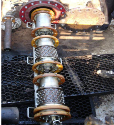
Fig. 8 – Wall thickness assessment device-MFL.
