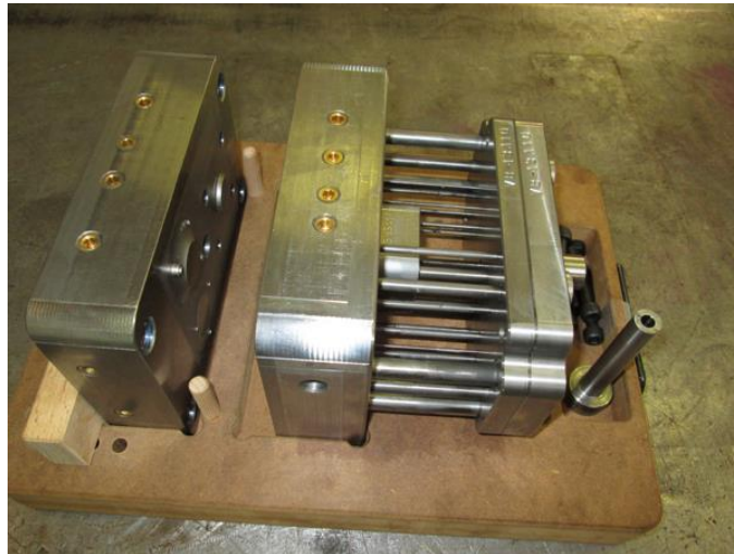
Fig. 1 – General structure of a Plastic Injection Mold
