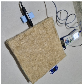
Fig. 5 – Measurement of the thermal conductivity and thermal capacity of the thermal insulation material.
