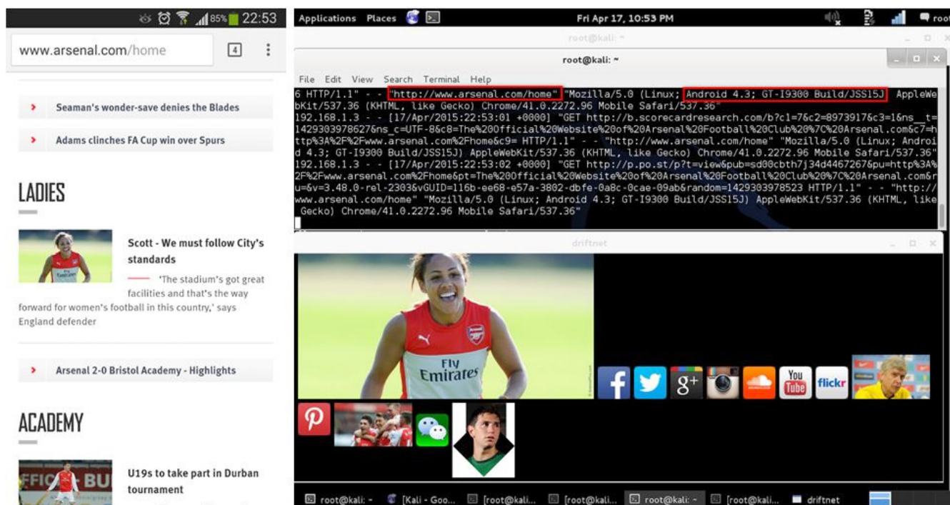
Figure 3: Comparison of the browser of a mobile user and display the captured traffic using URLsnarf and Driftnet tools Kali Linux (left mobile phone I9300, right Kali Linux tools)
