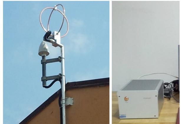
Figure 1: LINET field antenna (LFA), GPS antenna (left) and LINET field processor (LFP) (right)
