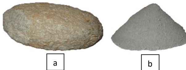
Figure 2. Perlite slag before borying (a) and 80 \mu\text{m} powder form (b).
