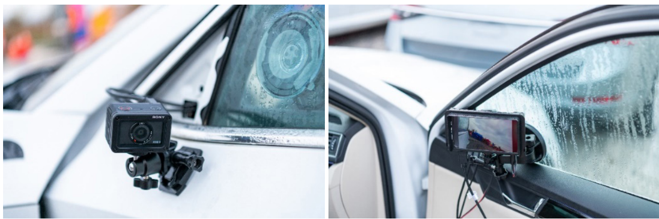
Fig. 3 Škoda Superb III modified to use DSM digital rear-view mirrors
