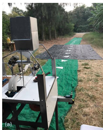
Fig. 2 (a) Experimental trials to determine the optimal angle; (b) Distribution of shrimp feed within a 15 m range angles of 25° and 55°
