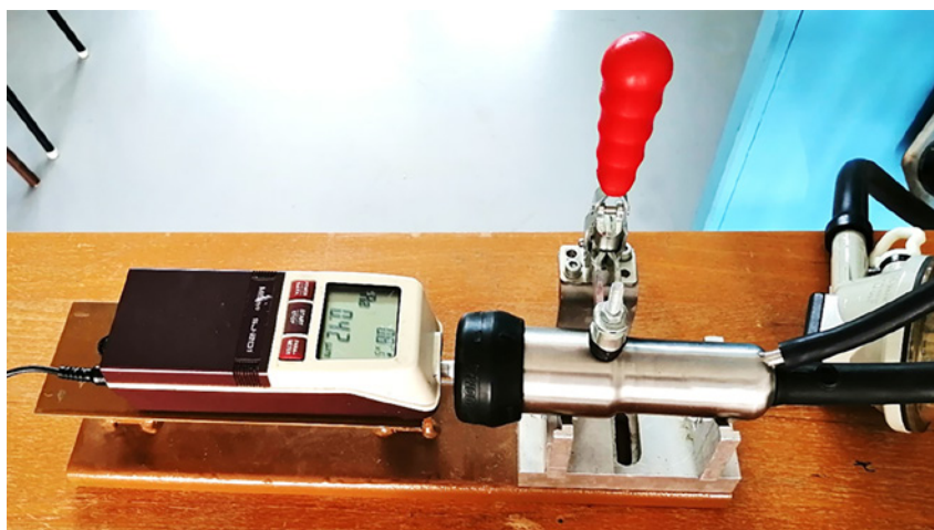
Fig. 3 Measuring bench for determining the roughness of the teat cup liner
