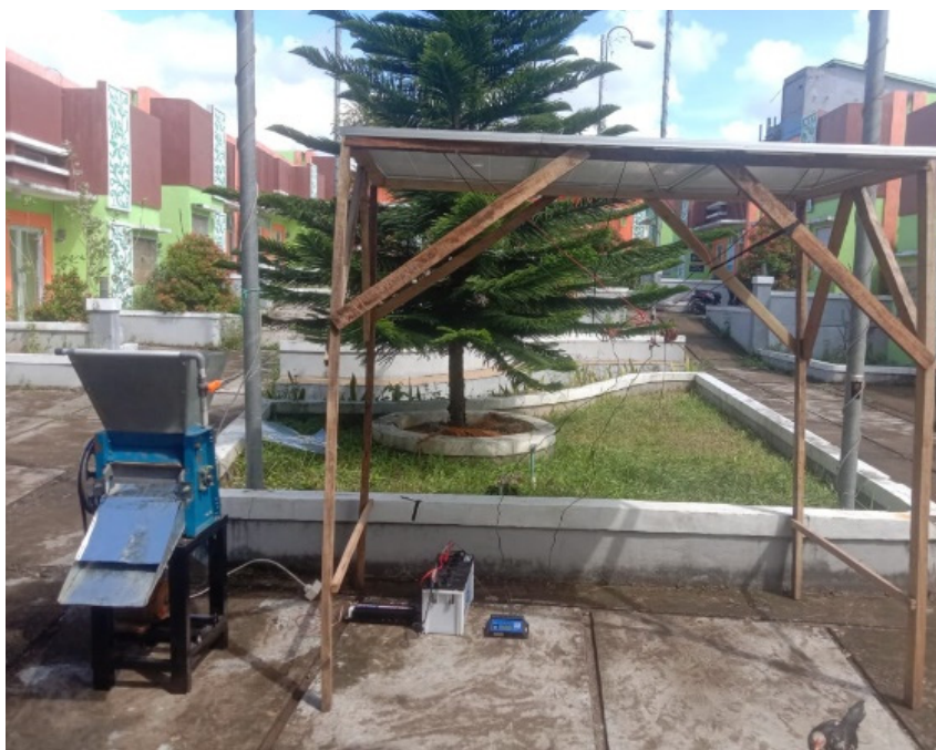
Fig. 4 Solar AC electric motor pulper
